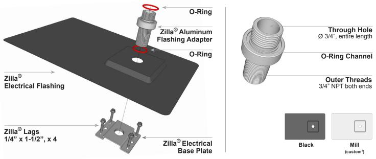
**Zilla<sup>®</sup> Electrical Flashing Assembly** is available in Black (ZEFLSH-A AL BLK) or custom colors<sup>1</sup> and includes: Electrical Base Plate, 4 mounting lags, Electrical Flashing, Aluminum Flashing Adapter and 2 O-Rings.
