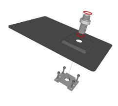
Side view of Assembly installed on Metal Roof showing Junction Box (not included)
