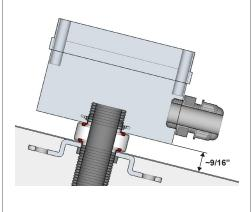
**Zilla<sup>®</sup> Electrical Flashing Assembly** is available in Black (ZEFLSH-AAL BLK) or custom colors<sup>1</sup> and includes: Electrical Base Plate, 4 mounting lags, Electrical Flashing, Aluminum Flashing Adapter and 2 O-Rings.
