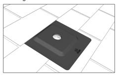
Keep the angle of the Flashing parallel with the roof so you don't disrupt the shingles or existing materials. Align the hole in the Flashing with the hole in the Base Plate.
