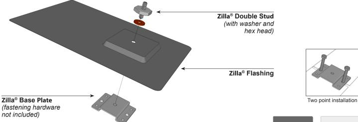
Zilla® Double Stud Flashing is available in Black (ZDSFA-15 AL BLK) or custom colors1 and includes: Double Stud with Encapsulated Gland Washer, Flashing and Base Plate. Zilla® Double Stud is a 3/8"-16 x 1-1/2" stainless steel stud with 3/16" recessed hex and 1-3/8" hex aluminum nut.
