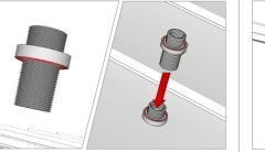
With an O-ring pressed in the channel on the underside against the metal roof insert the long end of the Adapter into the hole.
