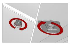
**NOTE:** Once the O-ring and Base Plate are in firm contact with the metal roof material, spin 1/4 turn to tighten.
