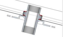
**3** Complete the Installation Attach components such as a Conduit Body or Junction Box as necessary.
