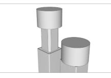
When the anchor is flush with the ground, or no more than two (2") inches above the ground, remove the Drive Cap.
