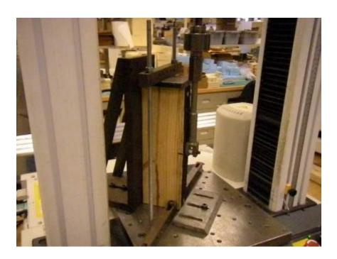
Photo No. 6 Zilla Zip Bolt - Setup for Lateral Loading
