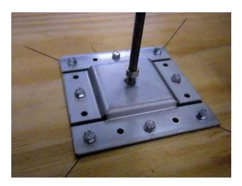
Photo No. 20 Double Stud XL Base Plate - Setup for Vertical Loading
