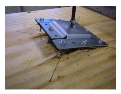
Photo No. 22 Double Stud XL Base Plate - Failure Detail for Vertical Loading
