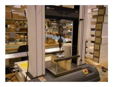
Photo No. 11 Double Stud Base Plate - Setup for Vertical Loading
