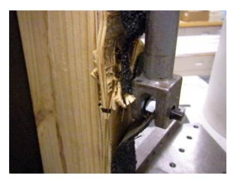
Photo No. 7 Zilla Zip Bolt - Failure Detail for Lateral Loading
