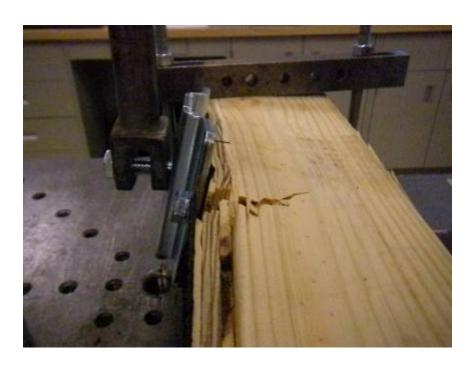
Photo No. 18 Double Stud Base Plate - Failure Detail for Lateral Loading (Perpendicular)
