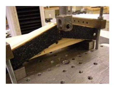
Photo No. 10 Zilla Zip Bolt - Failure Detail for Lateral Loading
