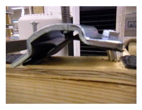
Photo No. 13 Double Stud Base Plate - Failure Detail for Vertical Loading
