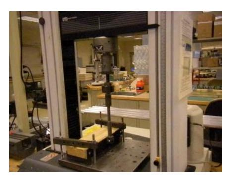
Photo No. 8 Zilla Zip Bolt - Setup for Lateral Loading (Perpendicular)
