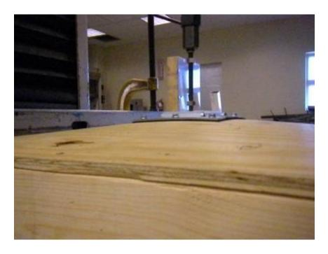
Photo No. 21 Double Stud XL Base Plate - Setup for Vertical Loading
