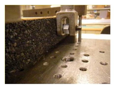
Photo No. 9 Zilla Zip Bolt - Setup for Lateral Loading
