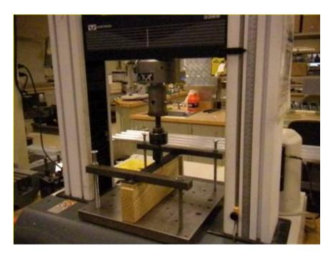
Photo No. 1 Zilla Zip Bolt - Setup for Vertical (Uplift) Loading
