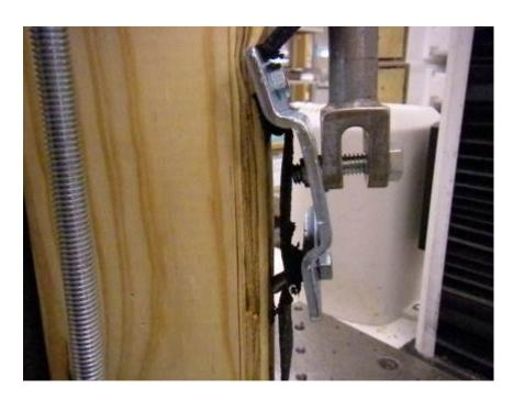
Photo No. 16 Double Stud Base Plate - Failure Detail for Lateral Loading (Parallel)
