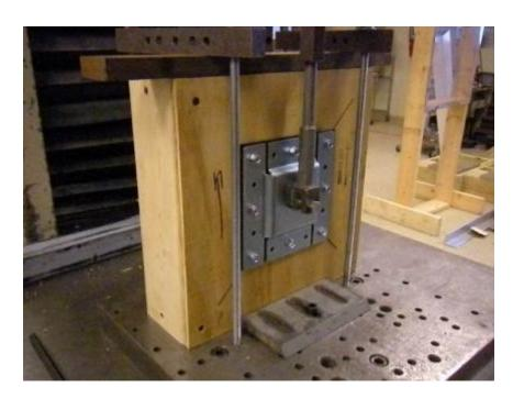
Photo No. 24 Double Stud XL Base Plate - Setup for Lateral Loading (Parallel)
