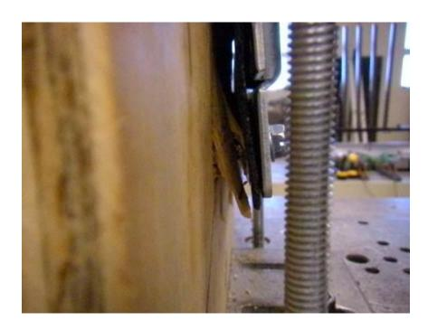
Photo No. 27 Double Stud XL Base Plate - Failure Detail for Lateral Loading (Perpendicular)
